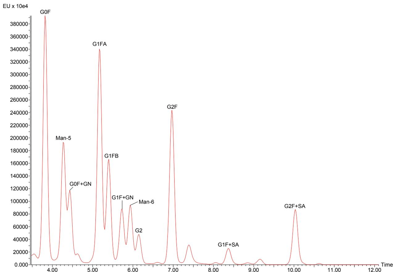
*Figure 5: The raw data obtained from HILIC-FLR analysis of the N-glycans released from a monoclonal antibody.*
