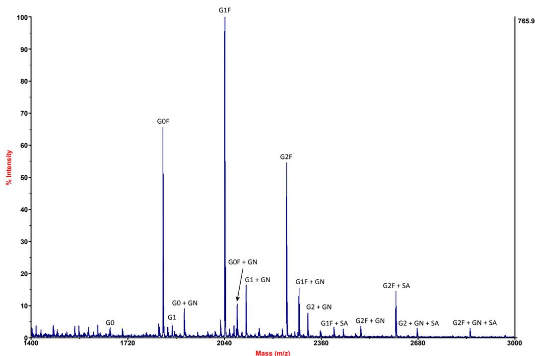
Figure 4: The raw data obtained from MALDI-TOF mass spectrometric analysis of the N-glycans released from a monoclonal antibody (the N-glycans were permethylated prior to analysis).
