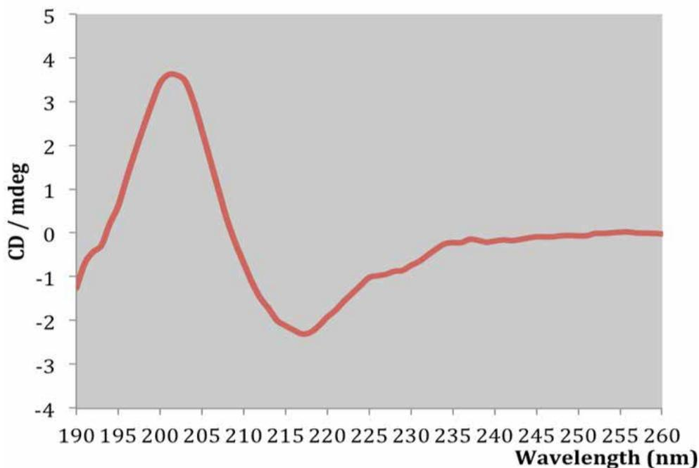
Figure 6: The raw data obtained from near-UV analysis of a monoclonal antibody
