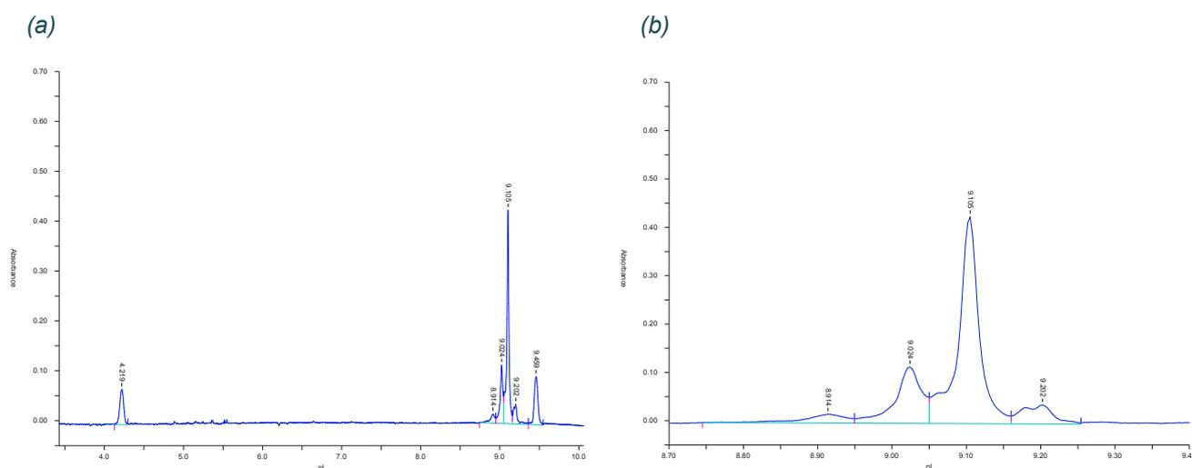
Figure 3: The UV (280nm) response across the capillary obtained following capillary isoelectric focusing of a monoclonal antibody by iCE3 (a) full electrophoretogram (the peaks around pI 4.2 and 9.5 are internal pI markers) (b) zoom of region of interest
