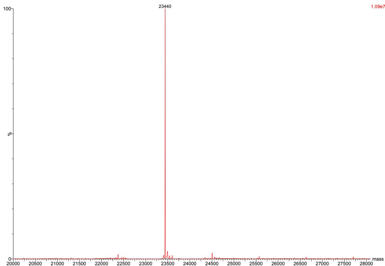
*Figure 2a: The deconvoluted mass spectrum obtained from on-line LC/ES-MS (Q-TOF) analysis of a monoclonal antibody following reduction. Average of the spectra acquired during elution of the released light chain.*
