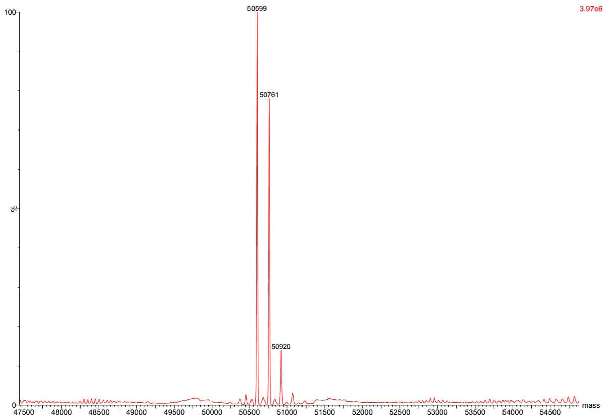
*Figure 2b: The deconvoluted mass spectrum obtained from on-line LC/ES-MS (Q-TOF) analysis of a monoclonal antibody following reduction. Average of the spectra acquired during elution of the released heavy chain.*
